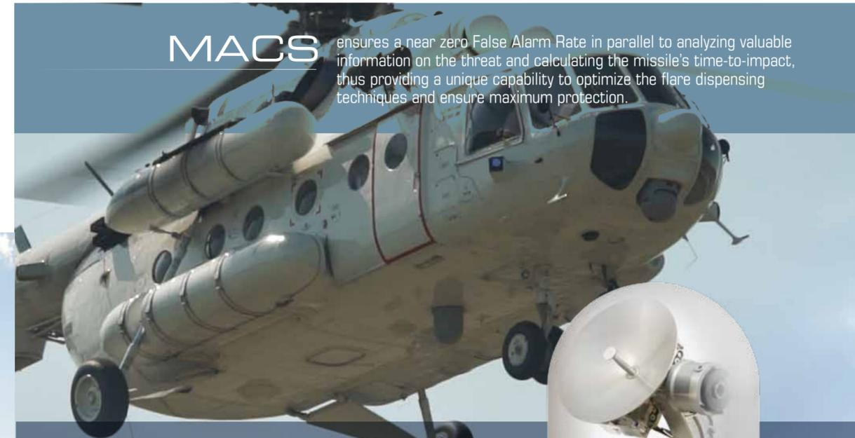
**MACS** ensures a near zero False Alarm Rate in parallel to analyzing valuable information on the threat and calculating the missile's time-to-impact, thus providing a unique capability to optimize the flare dispensing techniques and ensure maximum protection.
